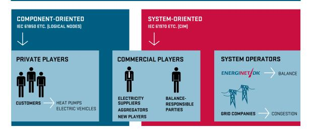
**COMPONENT-ORIENTED STANDARDS** (IEC 61850 etc.) are used when communicating with the customer's DER units, for example with an aggregator. The system-oriented standards (IEC 61970) are used among commercial players and in relation to the system operators.
